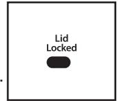
If you need to open the lid, press START/STOP/PAUSE/UNLOCK LID. The lid will unlock once the washer movement has stopped. This may take several minutes if the load was spinning at high speed. Press START/STOP/PAUSE/UNLOCK LID again to resume the cycle.
