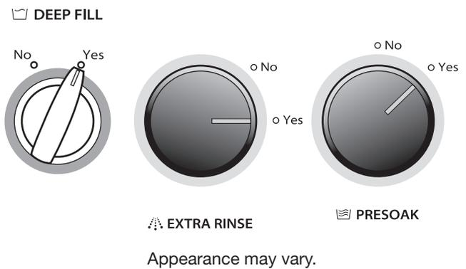
**Deep Fill:** Set at “Yes” to add extra water to your cycle. Water will be added automatically, with the amount determined by the size of the load.
