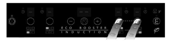
To change the power level, press the - / + buttons (from 1 to a maximum of 9). To deactivate the Flexi cook function, press simultaneously the 2 selecting buttons of the zones. To switch off the zones instantly, hold one of the zone selection button for 3 seconds.
