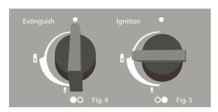
5. Turn the ignition Control Knob backwards to the " ● " position to extinguish the burner.
