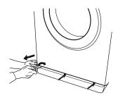
**7.** Container for the drained water: Place a low and wide container under the water filter in order to collect the residual water.
