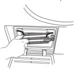
Clean the bottom filter under running water; wipe away dust and
