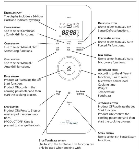
microwaves only and Combi functions. The button will not work with other functions.
