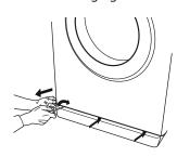
**7.** Container for the drained water: Place a low and wide container under the water filter in order to collect the residual water.
