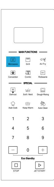
To cook with microwave power individually, press the Microwave button repeatly or press +/-button to select a cooking power level, press +/- or 0-9 keypad to set a desired cooking time. The longest cooking time is 90 minutes.
