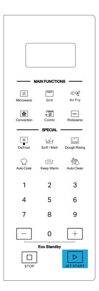
This feature allows you to start the oven quickly. Press JET START button once, the oven starts work at full power level automatically. During cooking, press JET START to add time. The longest cooking time is 90 minutes.
