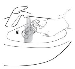
**6.** Insert the water filter and reinstall the kick panel: Re-insert the water filter by turning it clockwise. Turn it as far as it will go; the filter's grip should be in its vertical position. In order to check the filter's seal, pour about 1 litre of water into the detergent dispenser.
