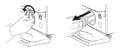
**5.** Clean the water filter: remove any residues from the filter and wash it under running water.
