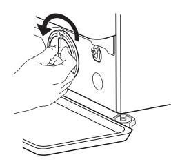
**4.** Remove the filter: Place a cotton cloth under the water filter in order to absorb any small amounts of residual water. Next, remove the water filter by turning it counter-clockwise.
