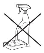
Do not use generic detergents, glass detergents, abrasive powders, or other similar products to clean the control panel, as these could damage the printed elements.
