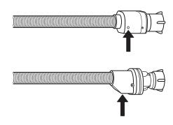
For flood protection hoses: check the safety valve's inspection window (see the arrow). If it's red, this means that the flood protection function has been engaged; in this case, the hose will have to be replaced with a new one. In order to detach the hose, press the release button (if present) and unscrew the hose.
