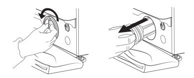
**5.** Clean the water filter: remove any residues from the filter and wash it under running water.
