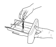
**3.** Wash the components under running water, taking care to remove all the detergent and fabric softener residues.
