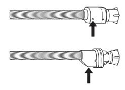
For flood protection hoses: check the safety valve's inspection window (see the arrow). If it's red, this means that the flood protection function has been engaged; in this case, the hose will have to be replaced with a new one. In order to detach the hose, press the release button (if present) and unscrew the hose.
