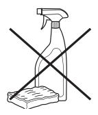
Do not use generic detergents, glass detergents, abrasive powders, or other similar products to clean the control panel, as these could damage the printed elements.
