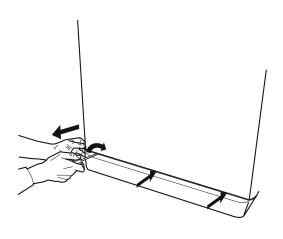
**2.** Container for the drained water: Place a low and wide container under the water filter in order to collect the residual water.
