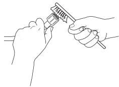
**3.** At this point, manually unscrew the intake hose from the back of the washer dryer. Using pliers, extract the mesh filter from the valve on the back of the washer dryer and clean it.
