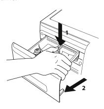
**2.** Remove the insert from the fabric softener compartment.
