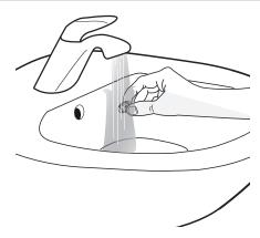
**4.** Re-insert the mesh filter. Reconnect the intake hose to the water tap and the washer dryer. Do not use tools to connect the intake hose. Open the water tap and check to make sure that all the connections have been tightened properly.
